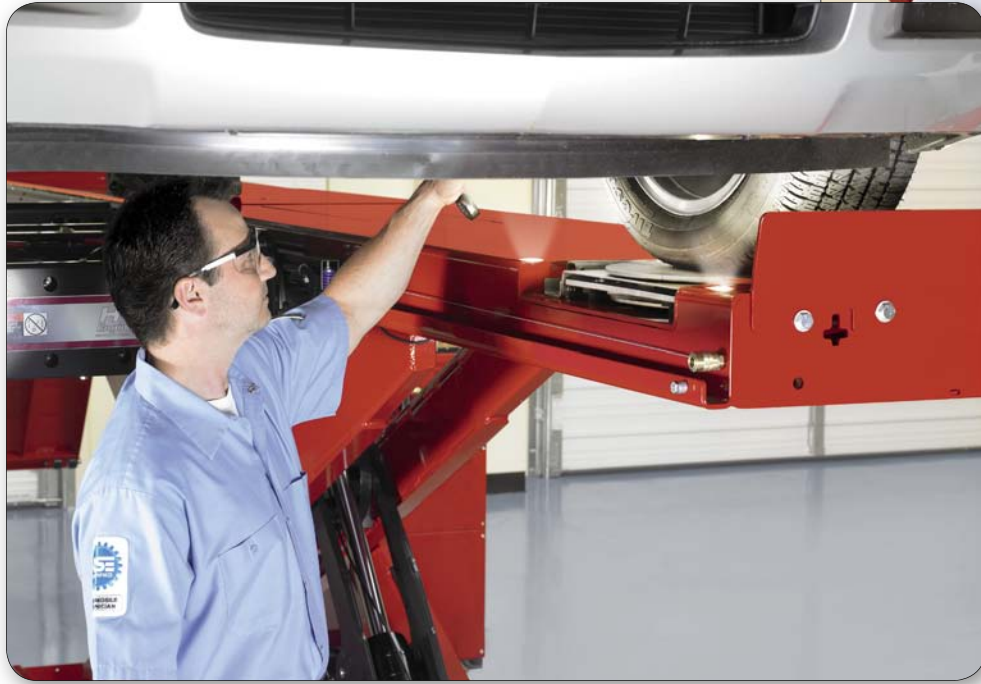
Above: Hunter's new 9,000-lb swing air jacks combine speed and power for ultimate ease of use.
